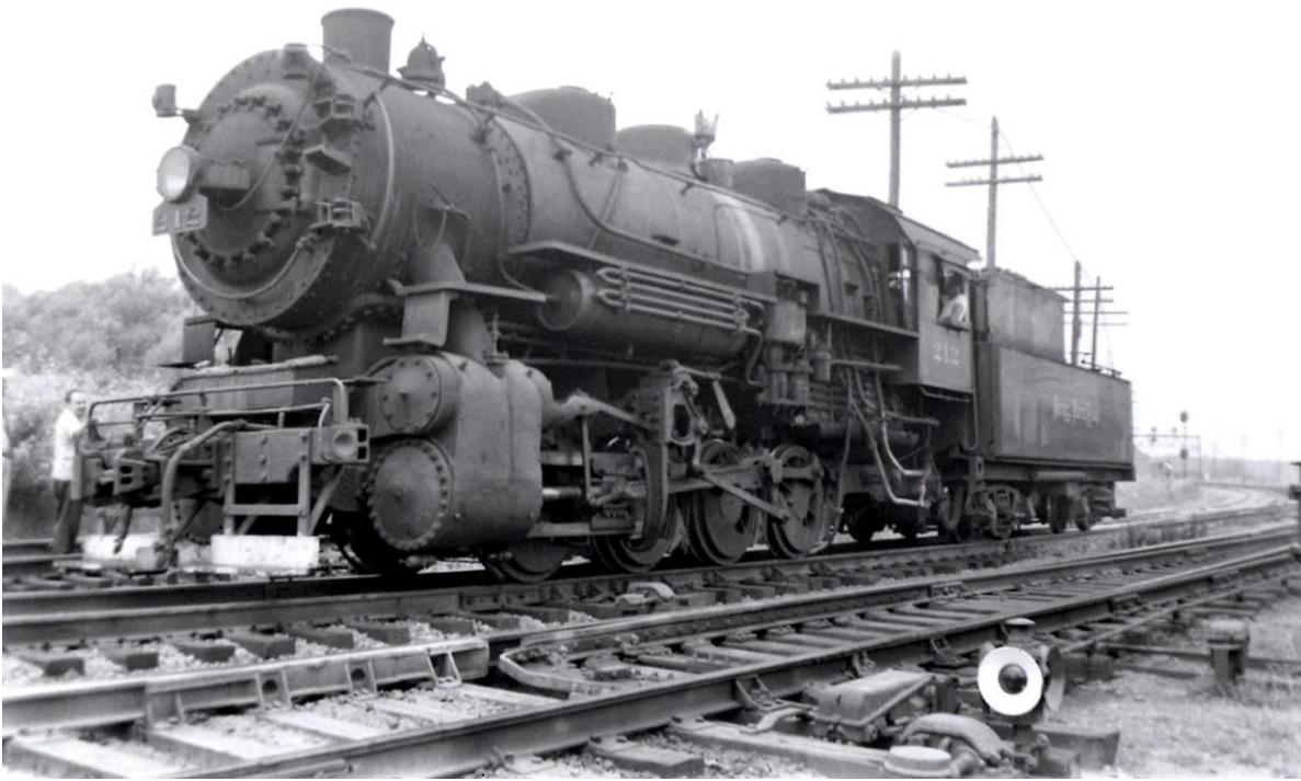
NKP #212 class U-3b 0-8-0 Switcher built by Lima, May 1924. Photo was taken opposite GB block station in Blasdell, NY on July 21, 1957
